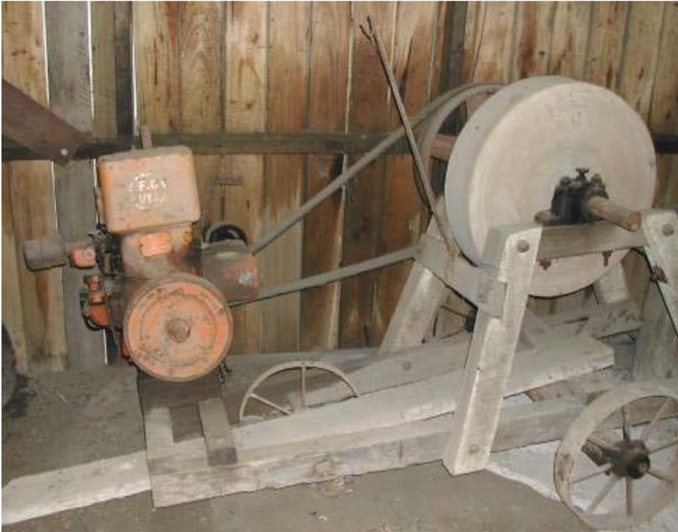
Plate 5: Portable motorised grind stone assumed to be for sharpening axes.
