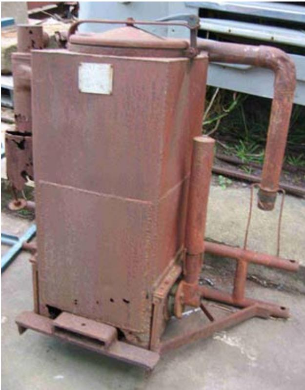
Plate 2: Kent gasifier from Horsham, a typical example of the basic charcoal gasifier design.
